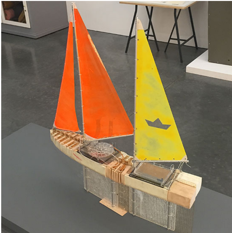
“Protei 010.9 Mini Cargo” by Cesar Harada, 2014. Acrylic, polycarbonate, EVA foam, stainless steel, 2 Towerpro MG95 Digi Hi Speed motors, 4 AA batteries, and nylon chord.
